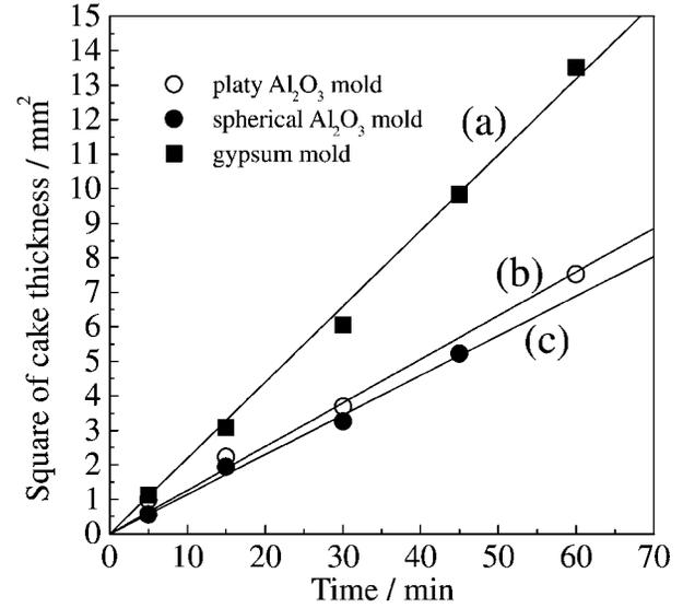
Figure 3 Relationship between the square of the thickness of green compact and casting time. (a) a gypsum mold, (b) a porous spherical mold, and (c) a porous platy mold.
