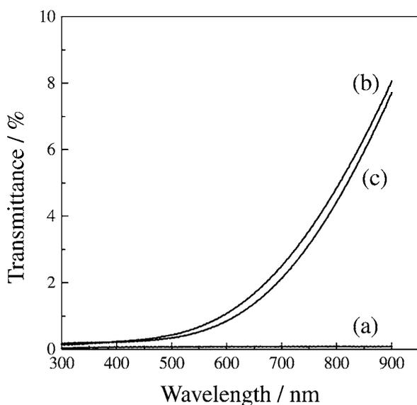
Figure 7 Transmittance of the sintered  $\text{Al}_2\text{O}_3$  compacts produced by slip casting using (a) a gypsum mold, (b) a spherical  $\text{Al}_2\text{O}_3$ -glass mold, and (c) a platy  $\text{Al}_2\text{O}_3$ -glass mold. The sample thickness was 1 mm.
