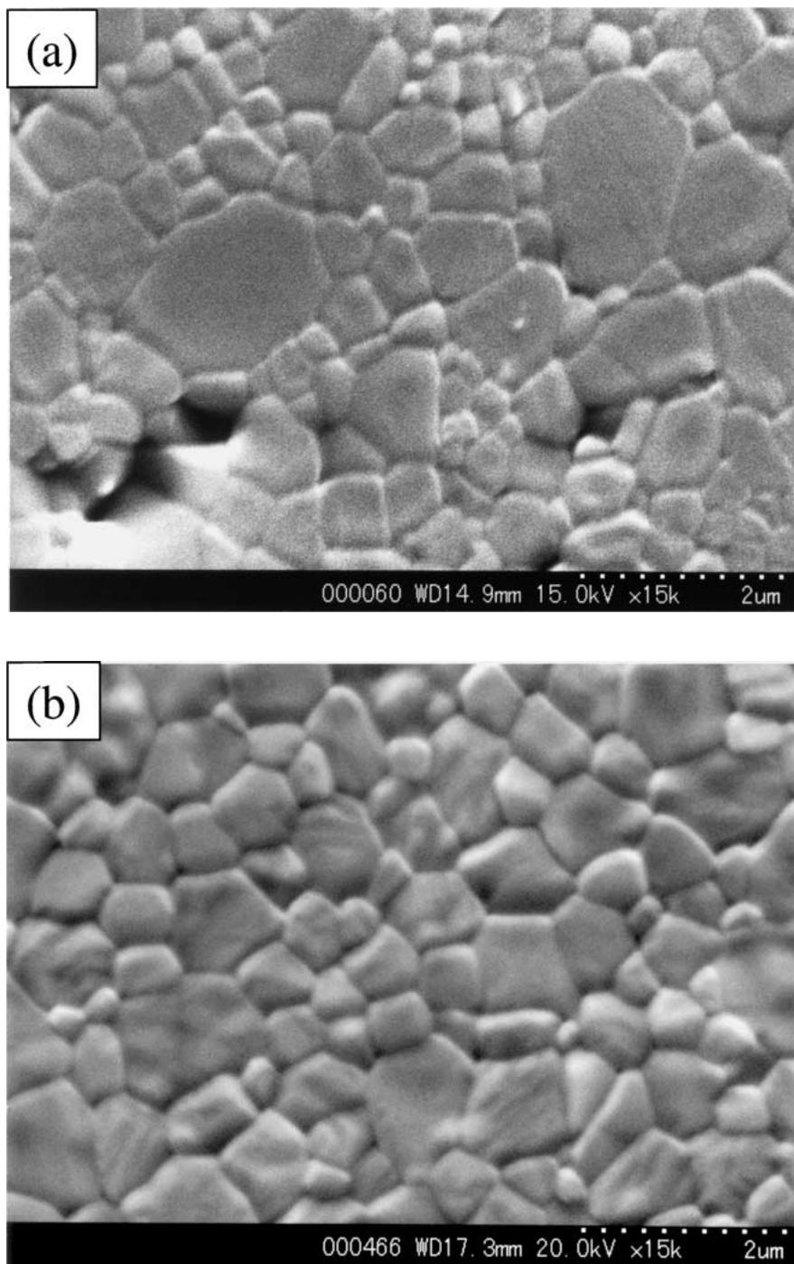
Figure 5 Microstructures of the  $\text{Al}_2\text{O}_3$  bodies sintered at  $1350^\circ\text{C}$  for 2 h under vacuum after slip casting using (a) a gypsum mold and (b) a porous  $\text{Al}_2\text{O}_3$ -glass mold.
