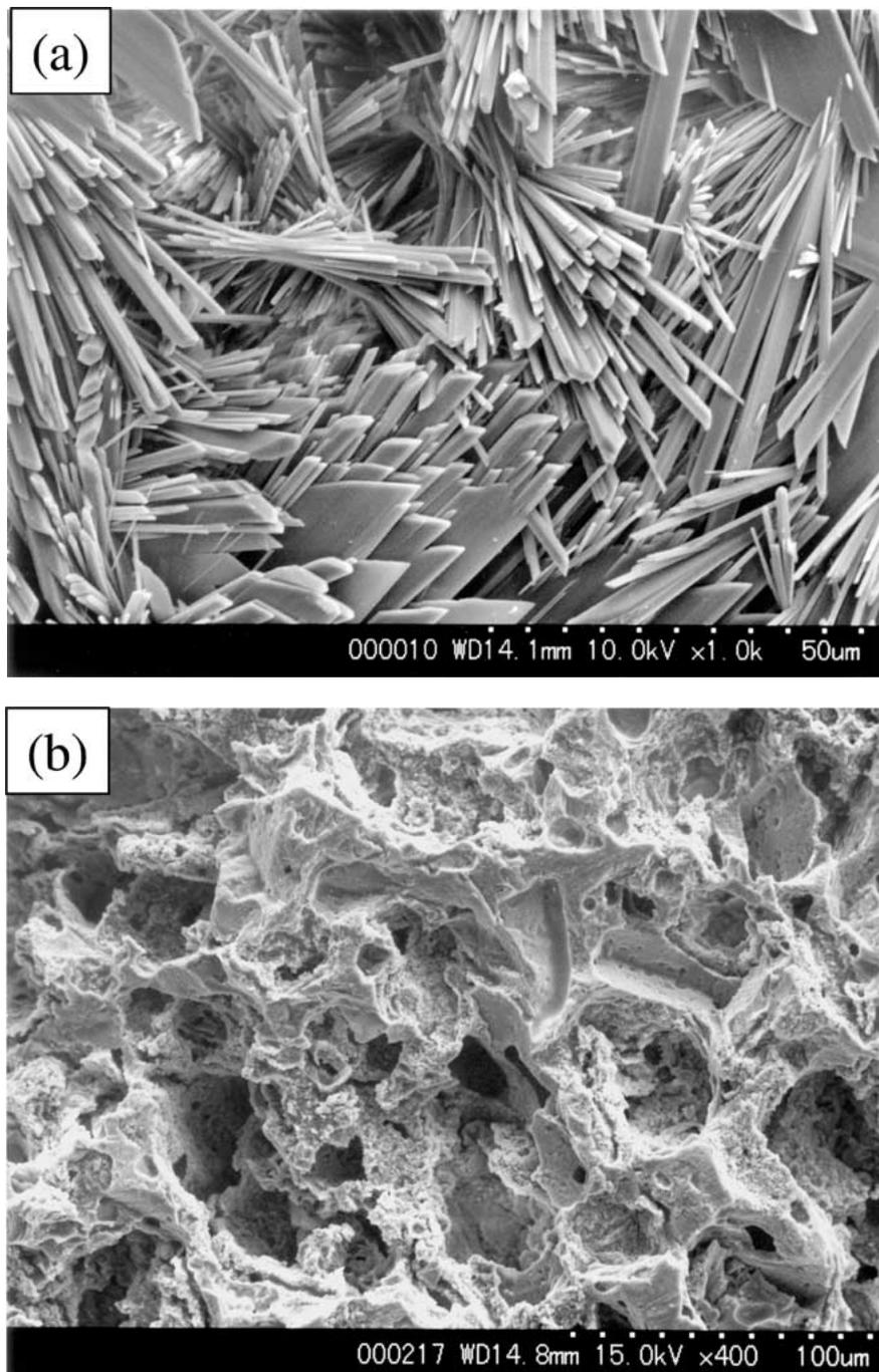
Figure 4 SEM images of fragments of (a) a gypsum mold, (b) a porous spherical  $\text{Al}_2\text{O}_3$ -glass mold and (c) a porous platy  $\text{Al}_2\text{O}_3$ -glass mold. (Continued.)
