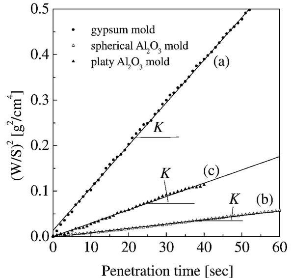
Figure 2 Relationship between the square of water absorption weight immersed into (a) a gypsum mold, (b) a spherical Al<sub>2</sub>O<sub>3</sub>-glass mold, and (c) a platy Al<sub>2</sub>O<sub>3</sub>-glass mold, (W/S)<sup>2</sup>, and penetration time.
