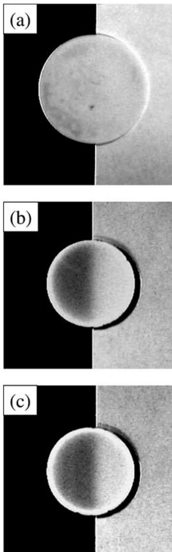
Figure 6 Photographs of the sintered compacts prepared by using (a) a gypsum mold and (b) a porous spherical  $\text{Al}_2\text{O}_3$ -glass mold, and (c) a porous platy  $\text{Al}_2\text{O}_3$ -glass mold.
