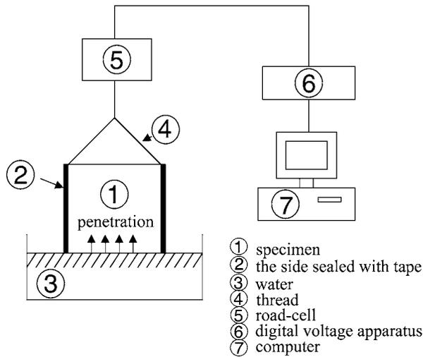
Figure 1 Scheme of the absorbed water experiments.
